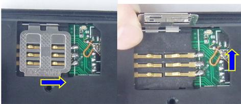
5.1.3 Put the SIM card into the holder, and turn the foil right and fasten it in place.
