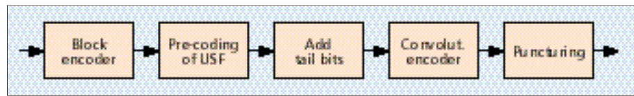
■ FIGURE 11. Encoding of GPRS data packets.
